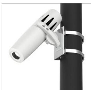
This weatherproof outdoor projector is equipped with the latest LED technology and is passively cooled without a fan. An external ballast is supplied, which is connected to the projector via waterproof cabling. PHOS 25 pole mount is suitable for year-round outdoor use or for damp interiors. The projector is especially suitable for outdoor projections on facades or portals, messages on pavements or areas in pedestrian zones. The projection motif (gobo) can be changed without tools.
